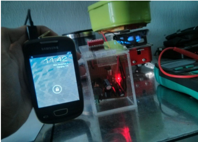
Figure 16 : Charging Smartphone by Using TEG Power Generation Device
