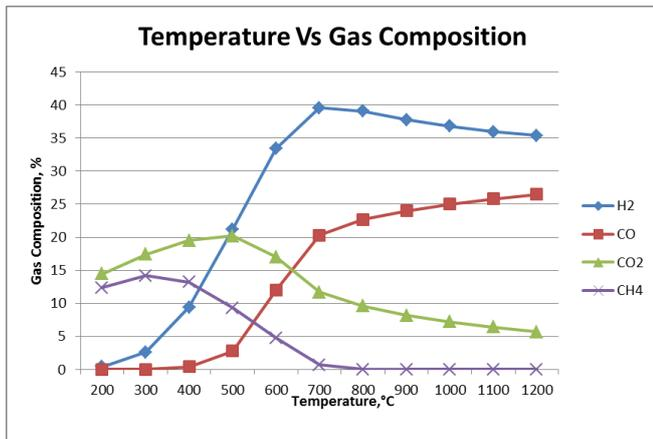
Fig. 7: Graph of gasification temperature versus gas composition
