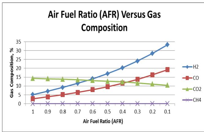
Fig. 9: Graph of Air Fuel Ratio (AFR) versus gas composition
