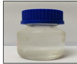
After the raw gas flow through condenser and two filter beds consist of sawdust and activated carbon. Another sample is taken. This is to know the effectiveness of the type of material use as a filter to trap the tar.
