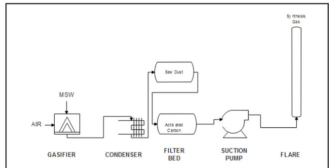
Fig. 3: Process flow diagram of pilot scale downdraft gasifier
