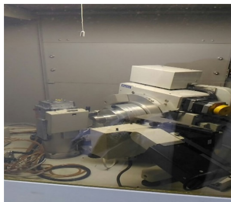
Figure 5. XRD used to determine new crystalline structure in cocrystals
