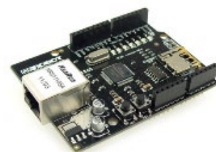
Fig. 6 Ethernet shield W5100
