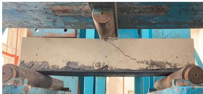
Figure 3 : Retrofitted RC beam with CFRP
