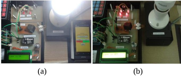
Figure 14. System Condition when (a) LampON Button and (b) LampOFF button is Pressed
