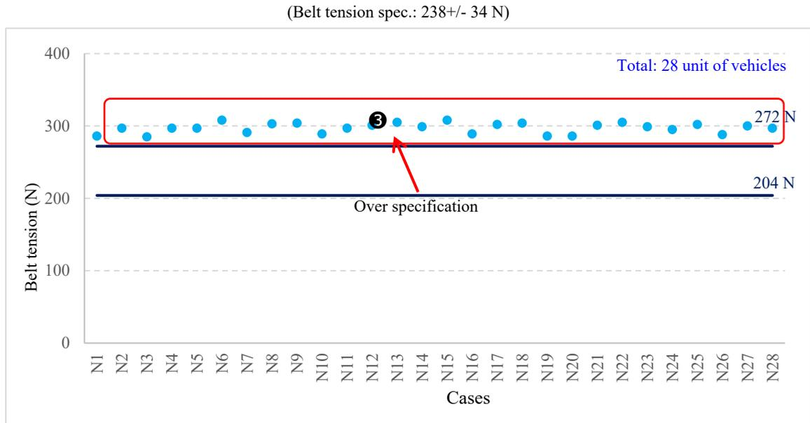
Fig. 6. New vehicles after quality control check by customer P Manufacturing.
