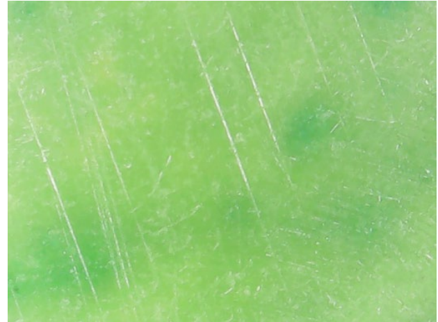
Figure 2: Simple micrograph of PES membrane before lipase immobilization at concentration of 2 mg/ml.
