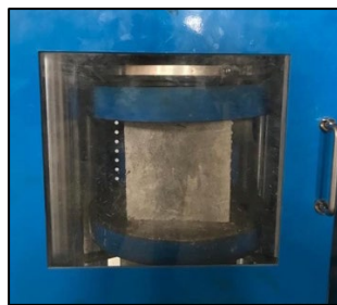
Figure 3. Compression test setup (BS EN 12390-3:2019, 2019)
