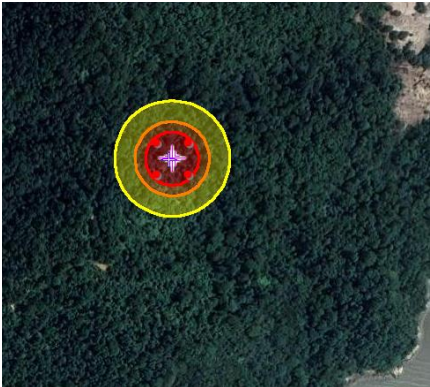
Figure 16. Fire by 50 mm Leak of Reactor at Plant 1
