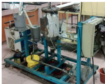
Fig 2 : Pyrolysis Unit for the conversion of EFB to biochar.
