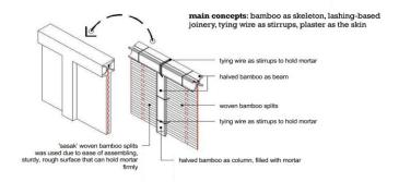
CONSTRUCTION DETAIL halved bamboo culms act as wall frame by positioning backside one to another, so the plaster can be filled into deep inside
