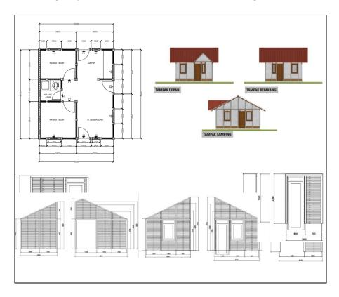
**Figure 1** Building plan and modules of plastered-bamboo wall panels. Image Copyright, Authors (2023)
