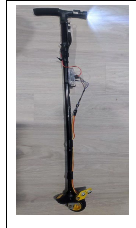
Figure 3. Innovation Blind sticks with LED and Ultrasonics Sensor
