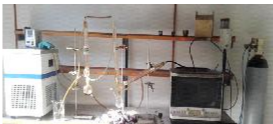
Fig. 1. Microwave apparatus for activated carbon regeneration
