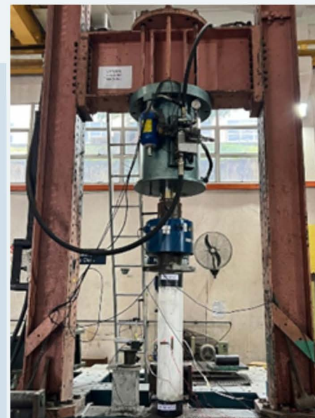
Figure 3. Experimental setup of RC column
