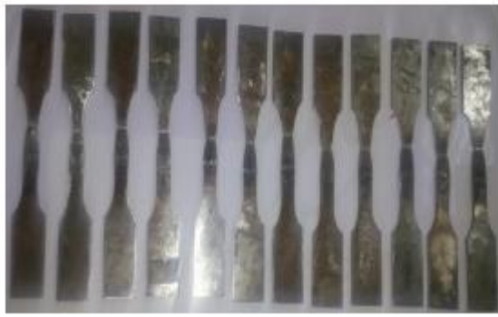
Figure 2.4: Broken Test Sample After Tensile Test
