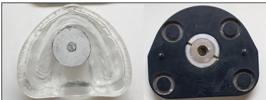
Figure 6: Metal attached on the epoxy substrate to substitute the non-retentive plastic fastener
