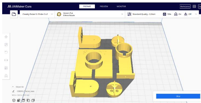
Figure 3.1: Designed solar tracker body parts STL file being transferred into UltiMaker Cura.
