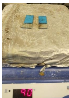
Figure 3: Annealing process of the FTO coated glass with \text{TiO}_2 and NiTsPc at 90^\circ\text{C} .
