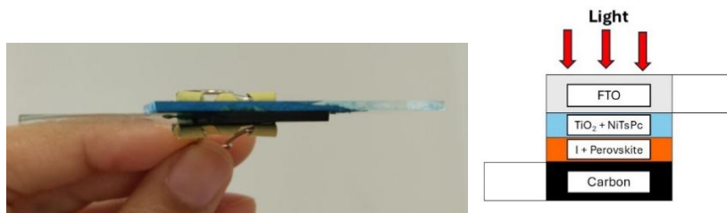
Figure 4: The attachment of surfaces of \text{TiO}_2 , NiTsPc, iodine, and perovskite onto carbon paste-FTO coated glass.
