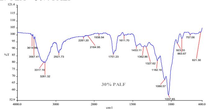
Figure 2: FTIR result for PLA + 30% PALF
