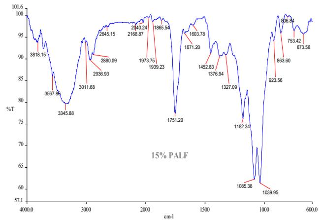
Figure 1: FTIR result for PLA + 15% PALF
