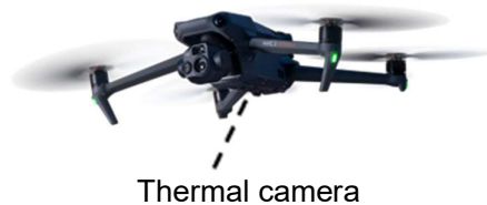
Figure 2. Thermal camera mounted on the DJI Mavic 3T.
