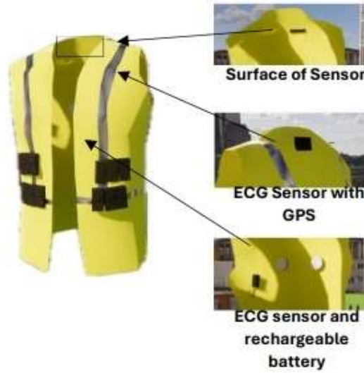
Figure 4 The component in body part of smart aid safety vest
