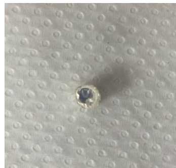
Fig. 1: The magnified view of the tin capsule to place the sample that was already being prepared in a powder form.
