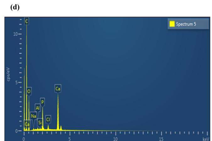
**Figure 3: SEM images of the HAp specimen after immersion in SBF for 25 days; (a) HAp with the size of 5 μm, (b) HAp with the size of 50 μm, (c) HAp with the size 100 μm, (d) EDX spectrum of HAp specimen after immersion in SBF for 25 days for the size of 100 μm**
