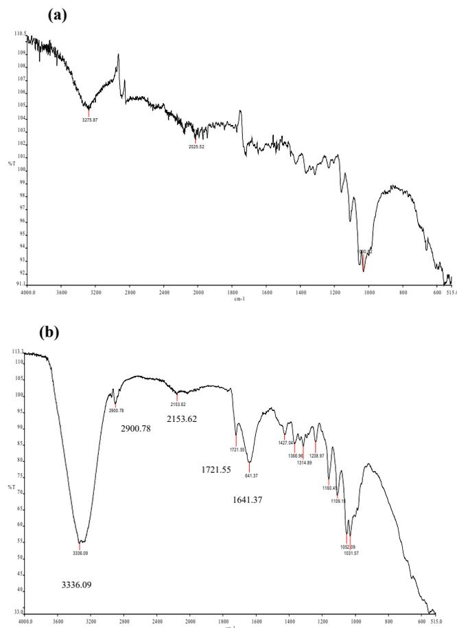
**Figure 1: FTIR Spectrum of HAp specimen; (a) before soaking in SBF, (b) after soaking in SBF for 25 days**
