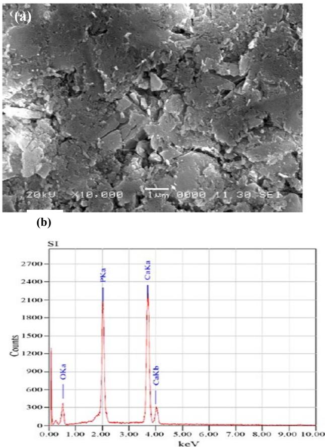
**Figure 2: (a) SEM image of pure HAp specimen before immersion in SBF, (b) EDX Spectrum of HAp specimen before immersion in SBF [11]**
