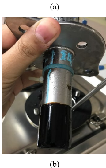
Figure 8: Changes of wax deposit surface and thickness with increasing temperature using MAC inhibitor at (a) 15°C (b) 5°C
