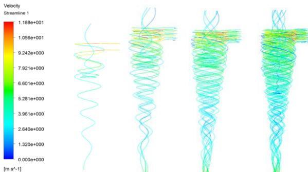
**Figure 5 : Streamline inside the cyclone**
