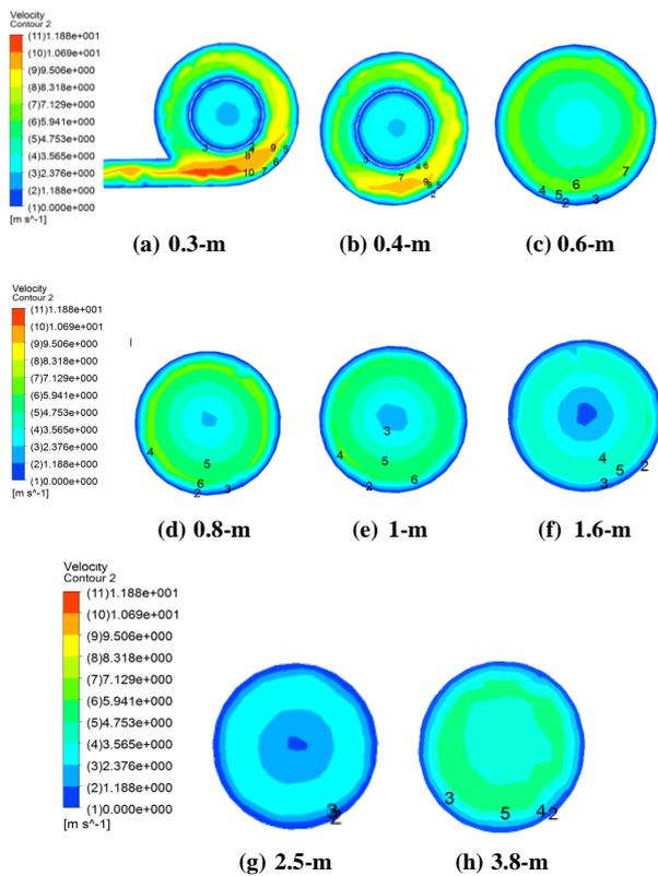
Figure 10 : Contours of velocity profiles from top of cyclone
