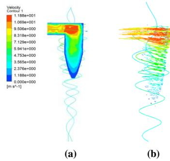
**Figure 6 : Contour for velocity magnitude at the inlet chamber**
