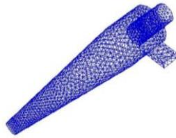
**Figure 1 : Meshing sketch of cyclone model**
