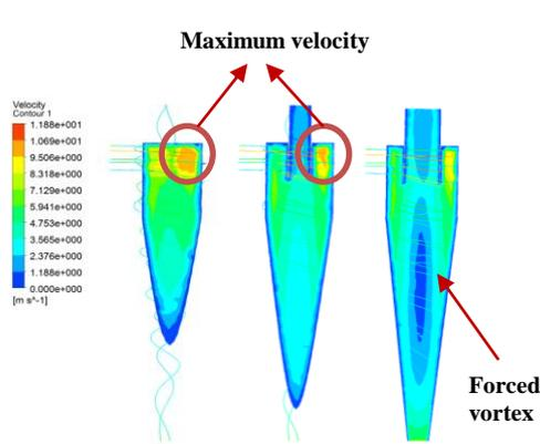
Figure 7a : Contour at -0.3-m, -0.2-m and 0-m from y-axis
