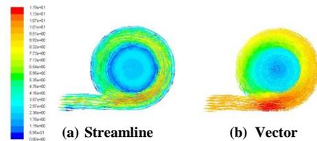
Figure 9 : Streamline and vector of fluid flow at vortex core
