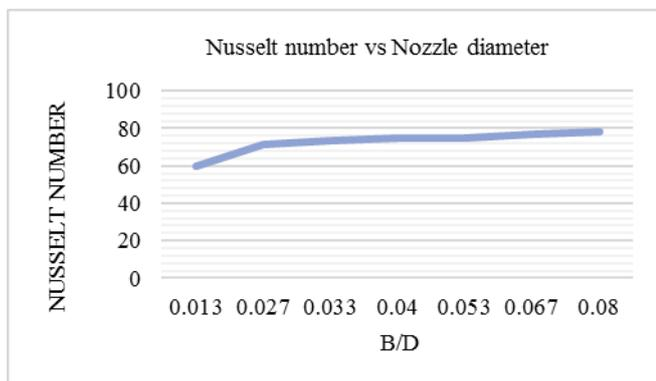
Figure 8 Effect of nozzle diameter on Nusselt number
