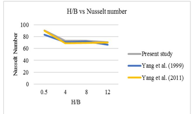
Figure 4 comparison of average Nusselt number distribution with Yang et al. [2] and Yang et al. [5]
