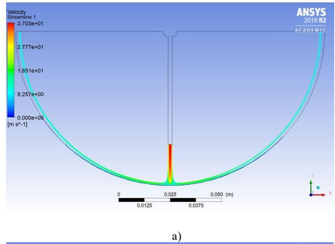
Figure 5 velocity vector of  $q'' = 5663 \text{ W/m}^2$ ,  $H/D = 0.13$ , (a)  $B/D = 0.013$ ; (b)  $B/D = 0.08$
