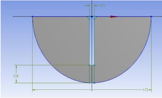
Figure 2 geometry of concave surface in Design Modeler (L11 = 6mm, L13 = 150mm and L14 = 20mm).
