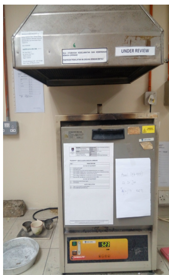
Fig 7: The furnace for the ash content of pulp
