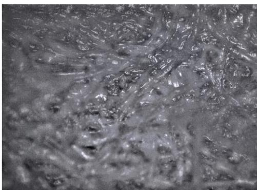
Figure 8: Surface of barium sulfate scale plate after dissolution.
