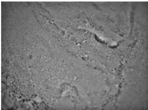
Figure 7: Surface of barium sulfate scale plate before dissolution.
