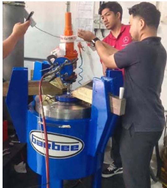
Figure 1-2: Internal test for safety relief valve
