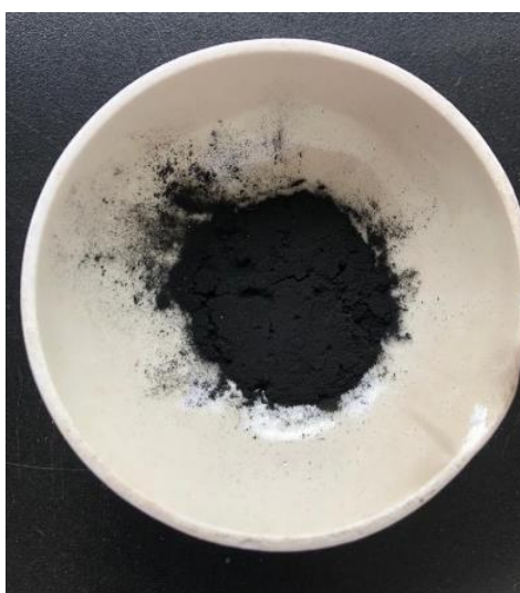
Figure 5. Activated carbon after heated at 500°C
