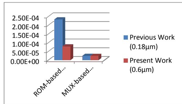
Figure 8: Average Power Consumption Vs Type of Encoder
