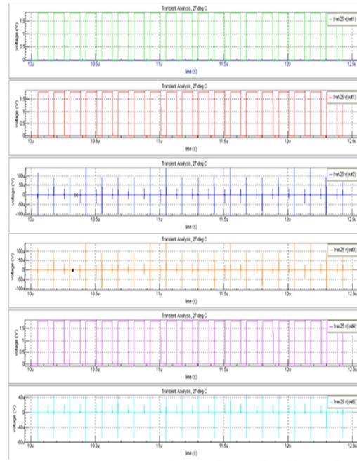
Figure 10: Transient Simulation of ROM-based Encoder
