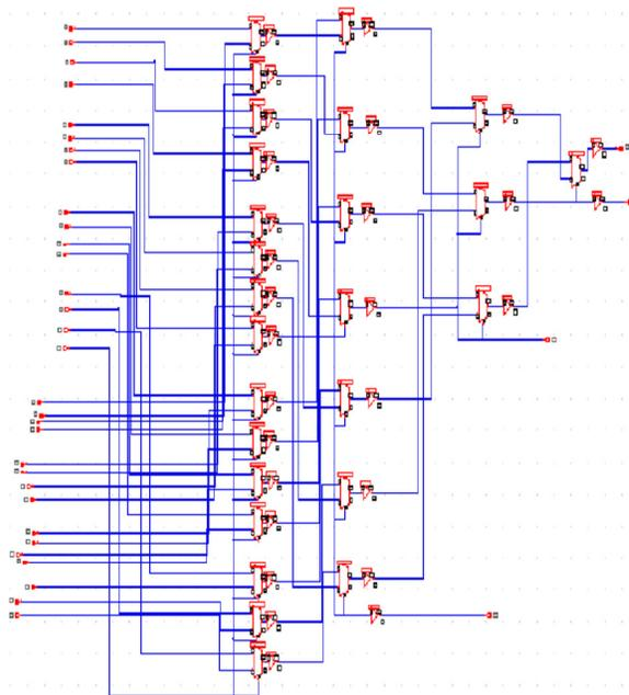
Figure 6: 5-Bit MUX-based Encoder
