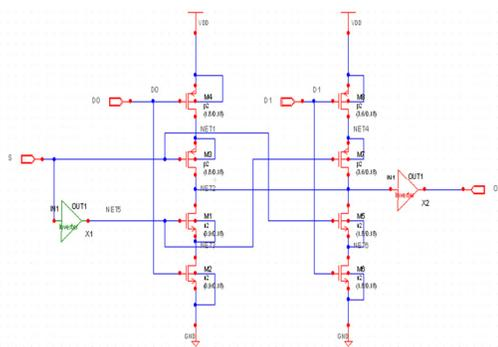
Figure 7: Static CMOS MUX
