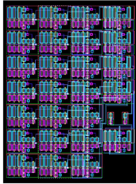
Figure 14: MUX-based Encoder Layout
