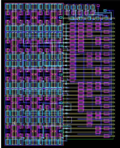
Figure 13: ROM-based Encoder Layout
