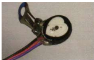
Figure 4: Pulse sensor with clip for putting it at earlobe
