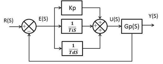
Figure 4. Parallel PID control structure
