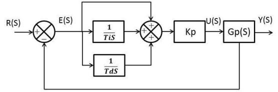
Figure 5. Ideal PID control structure
