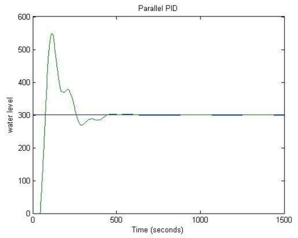
Figure 17. Parallel PID (ZN fine tuning)
