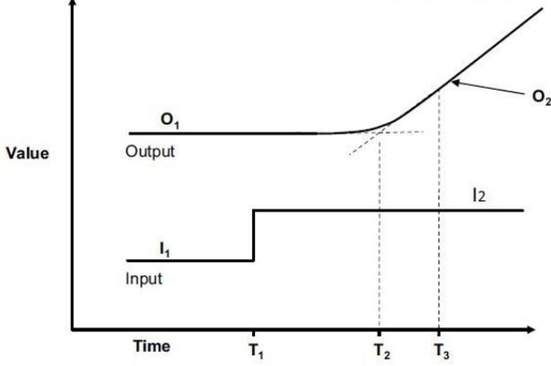
Figure 3. Response of integrating process
