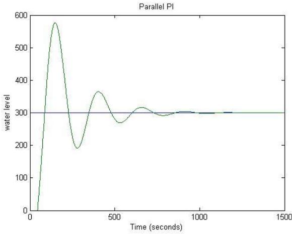
Figure 8. Parallel PI(ZN tuning)
