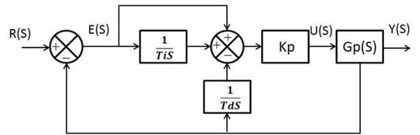
Figure 6. Alternative PID control structure
