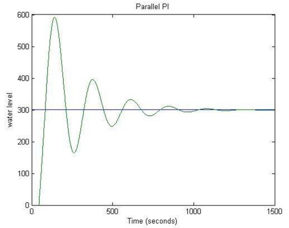
Figure 11. Parallel PI (ZN fine tuning)
