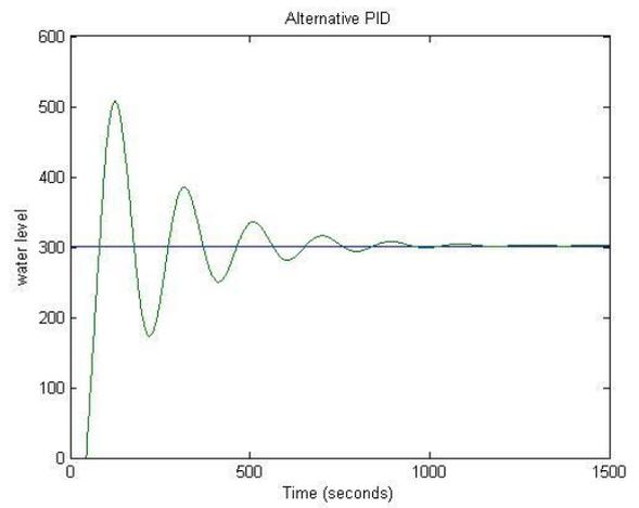
Figure 19. Alternative PID (ZN fine tuning)
