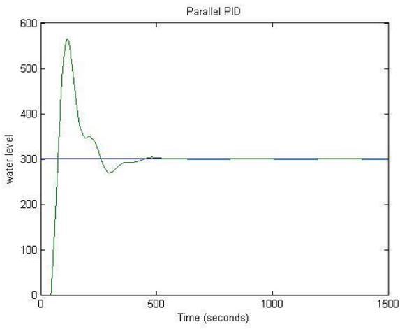
Figure 14. Parallel PID (ZN tuning)
