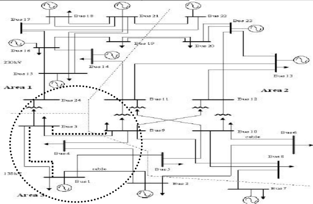
Figure4. Reliability 24 transmission bus system with double circuit transmission line
