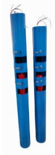
Fig. 8. Downstream sensor pole
