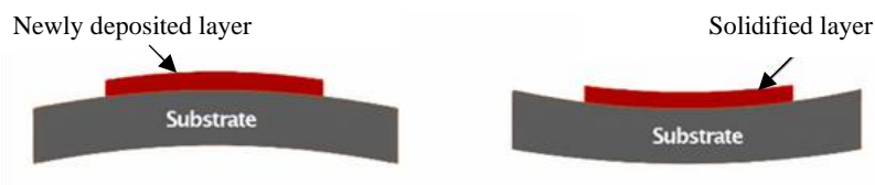
Fig. 1. The schematic diagram of distortion during the LMD process.
