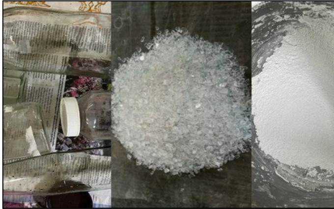
Figure 3: Process preparation of soda lime silica
