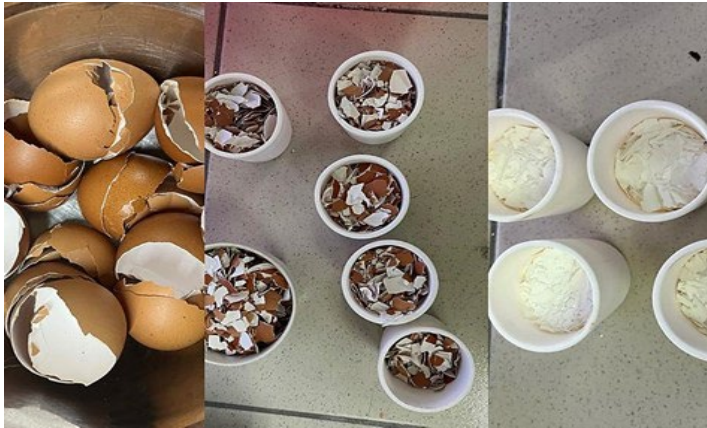
Figure 2: Process preparation of eggshells
