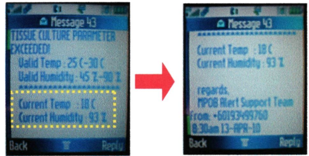
Figure 11(a) : The format of SMS notification when both temperature and humidity are exceeded
