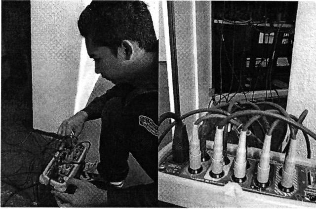
Figure 2: Installation using Fluke meter 1750
