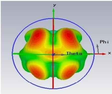
Figure 5(b).3D radiation pattern of round corners Vivaldi antenna
