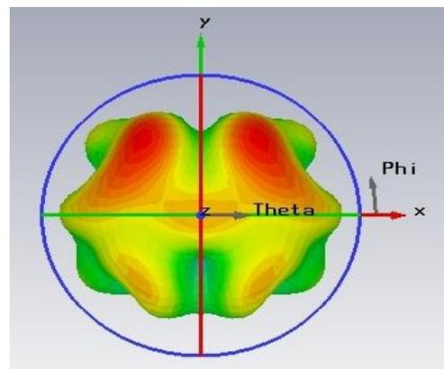
Figure 5(a). 3D radiation pattern of simple Vivaldi antenna
