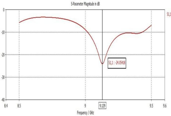
Figure 3(b).Simulation result of round corners Vivaldi antenna
