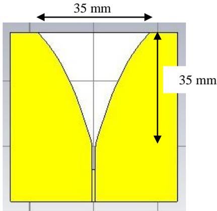
Figure 1. The design of tapered slot Vivaldi antenna
