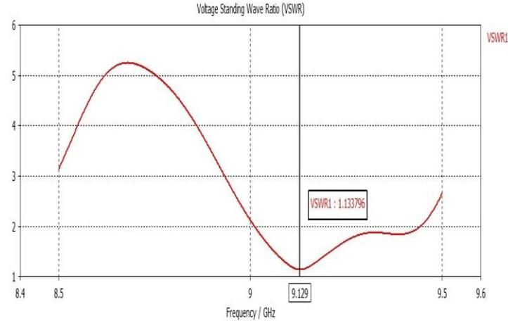
Figure 4(b).Simulation of VSWR of round corners Vivaldi antenna
