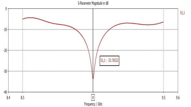
Figure 3(a). Simulation result of simple tapered slot Vivaldi antenna
