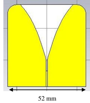
Figure 2. The design of round corners Vivaldi antenna
