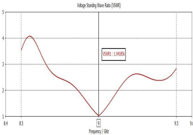
Figure 4(a).Simulation of VSWR of tapered slot Vivaldi antenna
