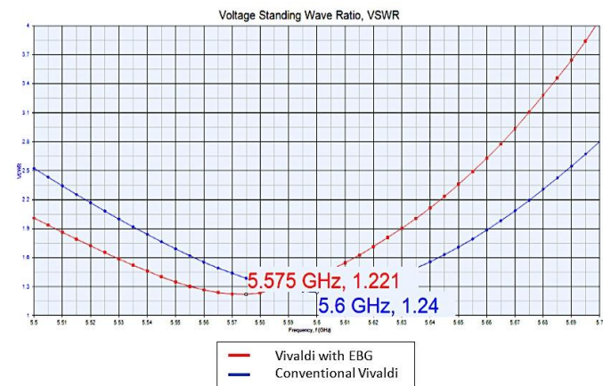
Figure 14: Measurement result of VSWR for Vivaldi antenna with and without EBG structure.
