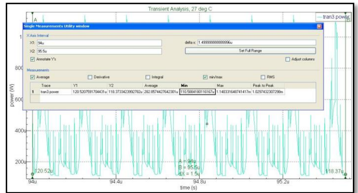
Figure 10: Average dynamic power dissipation for two stage opamp
