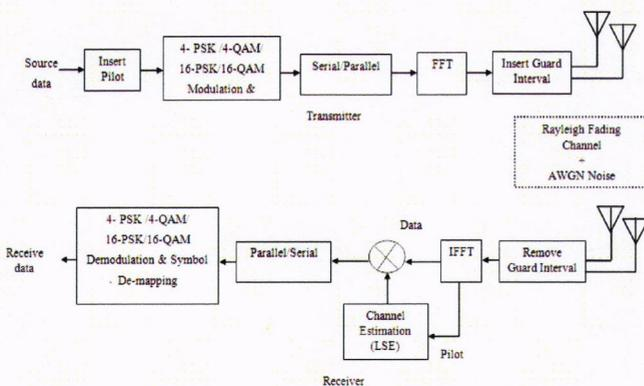
Figure 2: Block Diagram of MIMO-OFDM System.
