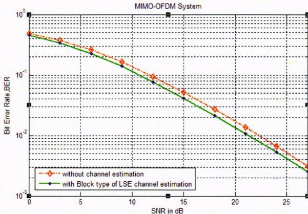
Figure 6: Comparison without channel estimation and with channel estimation.
