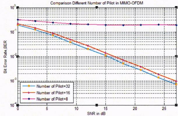
Figure 7: BER LSE of Block Type under Different Number of Pilot
