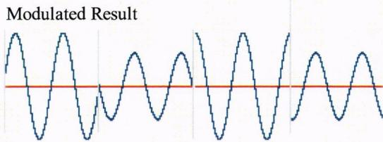
Figure 5: Digital Quadrature Amplitude Modulation (QAM).
