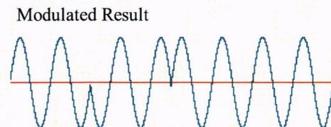
Figure 4: Digital Phase Shift Keying (PSK).
