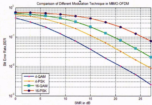
Figure 8: BER LSE of Block Type under Different Digital Modulation
