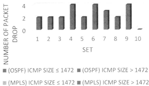
Figure 18: Number of Packet Drop for OSPF and MPLS without DF Bit Set (MTU = 1500)
