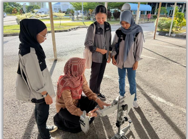
Students are listening to the facilitator's explanation regarding the British Pendulum Tester, an equipment used for skid resistance tests.
