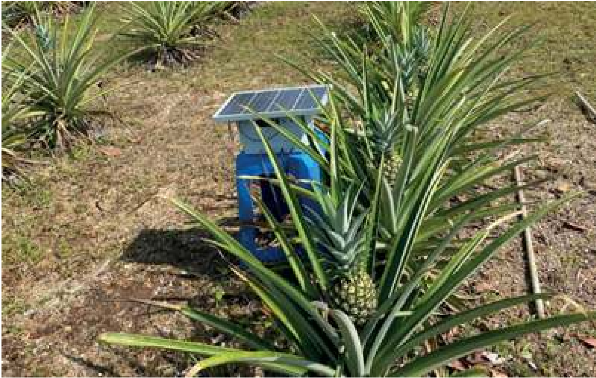
Figure 5.6 Application Of AASAS For Monitoring Soil Nutrient In The MD2 Pineapple Plantation
