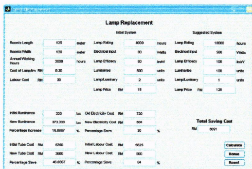
Figure 10: Matlab GUI program shows the costs that can be reduced by use the suggested lighting design
