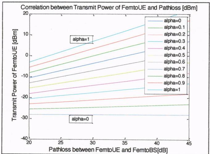
Figure 5. Correlation between Transmit Power and Path Loss (for different values of alpha,  $\alpha$ )
