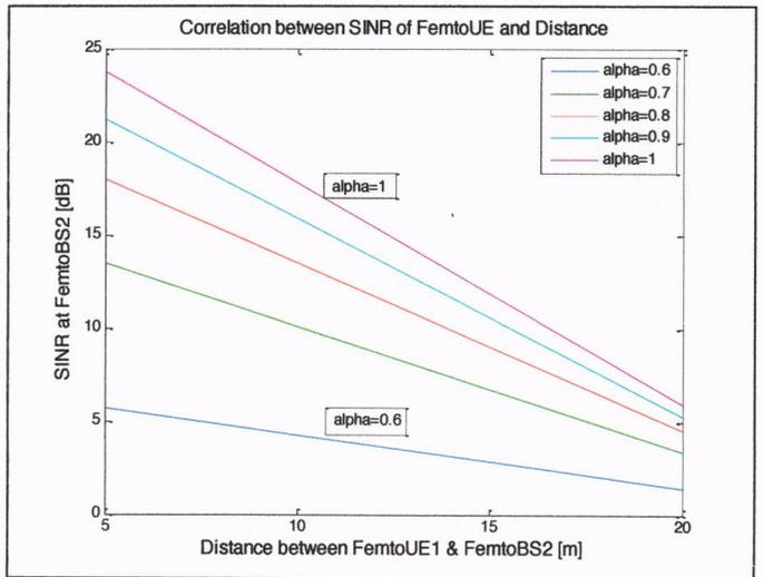
Figure 6. Correlation between SINR at FemtoBS and Distance from FemtoUE to FemtoBS
