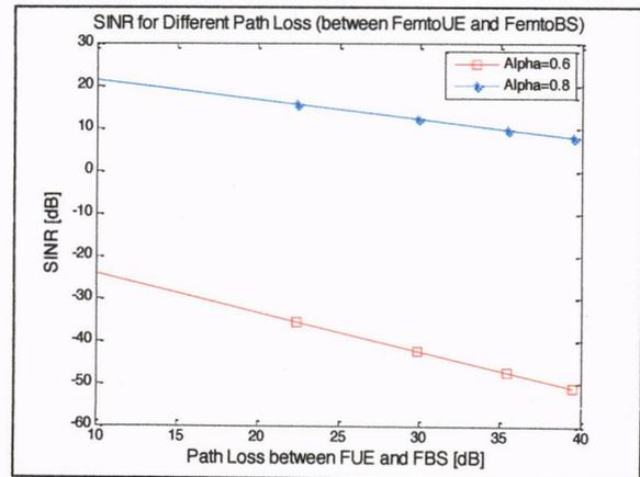
Figure 7. Correlation between SINR and Path Loss with varies of distance, d (alpha,  $\alpha = 0.6$  &  $0.8$ ) - using FPC equation
