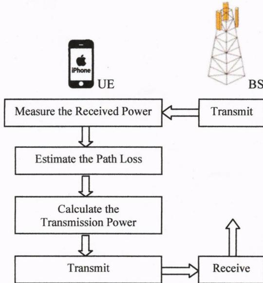
Figure 3. Block diagram of steps involved in setting the uplink power using the open-loop control
