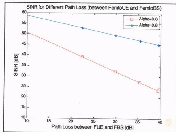
Figure 8. Correlation between SINR and Path Loss with varies of distance, d (alpha,  $\alpha = 0.6$  &  $0.8$ ) - using Propose/APC equation
