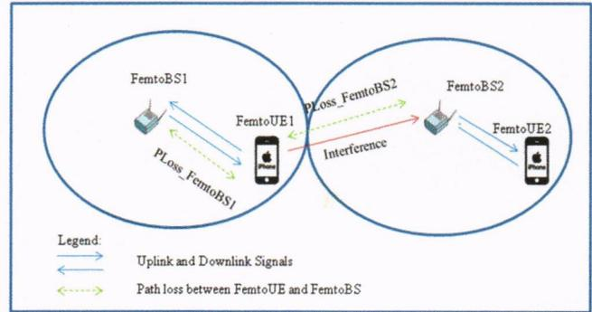
Figure 4. Interference Case 1 (FemtoUE to FemtoBS)
