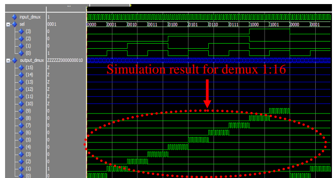
Fig. 7. Simulation Result for Demux 1:16
