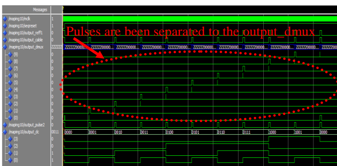
Fig. 13a. Pulse are been Separated to Output_Dmux
