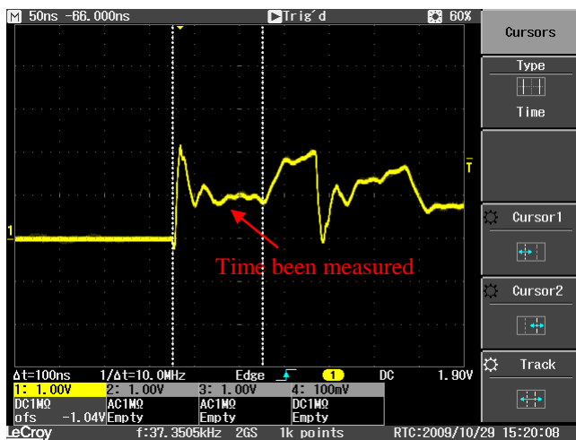
Fig. 17. TDR Measured Result and Pattern for Healthy Cable (100ns)
